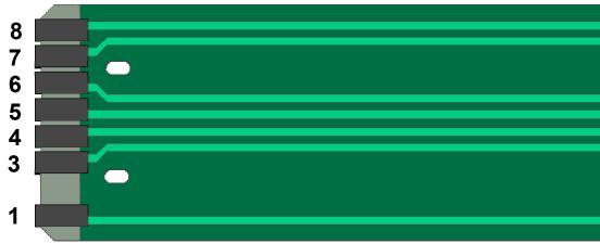
Depress Keyboard pad and test for continuity at all 3 test points.
