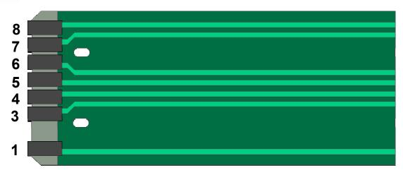
Depress Keyboard pad and test for continuity at all 3 test points.
